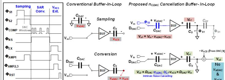
Figure 25.6.2: Circuit diagram of the proposed NS-SAR and the noise-mitigated buffer-in-loop technique.
