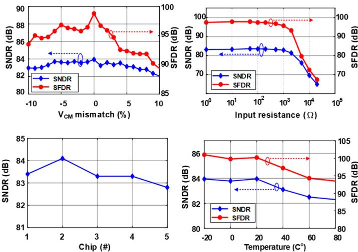
Figure 25.6.5: Measured SNDR/SFDR across V<sub>CM</sub> mismatch, input resistance, chip samples and temperature variation.
