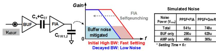
Figure 25.6.3: Proposed dynamic-biased PPSF with FIA assisted noise reduction.
