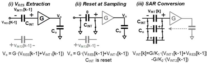
Figure 25.6.1: Signal flow of the proposed EF-CRFF architecture and D-amp-assisted integrator operation.
