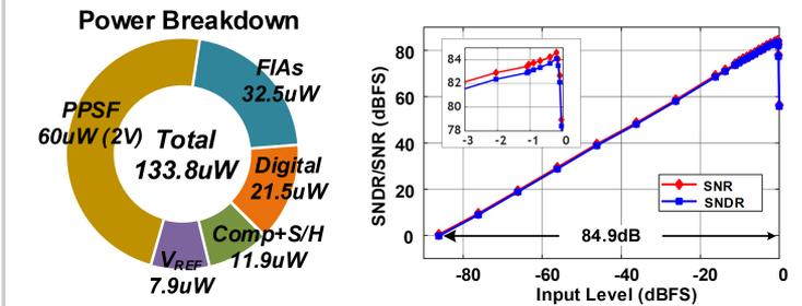
Figure 25.6.4: Measured output spectrum, power breakdown and dynamic range.
